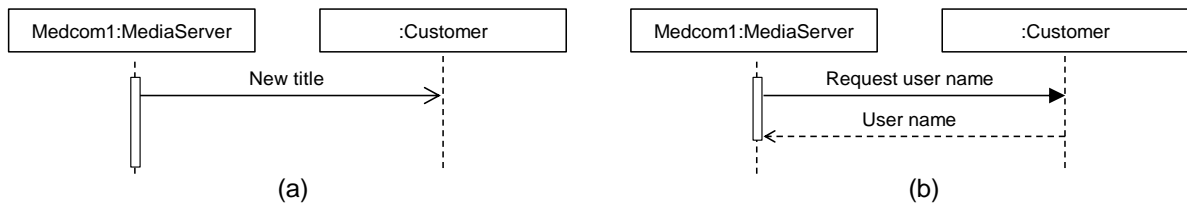
Figure 81: Modeling a) asynchronous and b) synchronous messages
